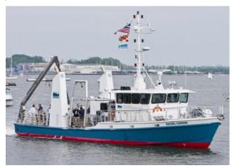
The *Carson* has been used to collect water quality samples; to tow plankton nets; to conduct box coring operations; to deploy a data buoy; to ground truth aircraft deployed instruments and as a platform to teach undergraduate and graduate students estuarine sampling techniques.
